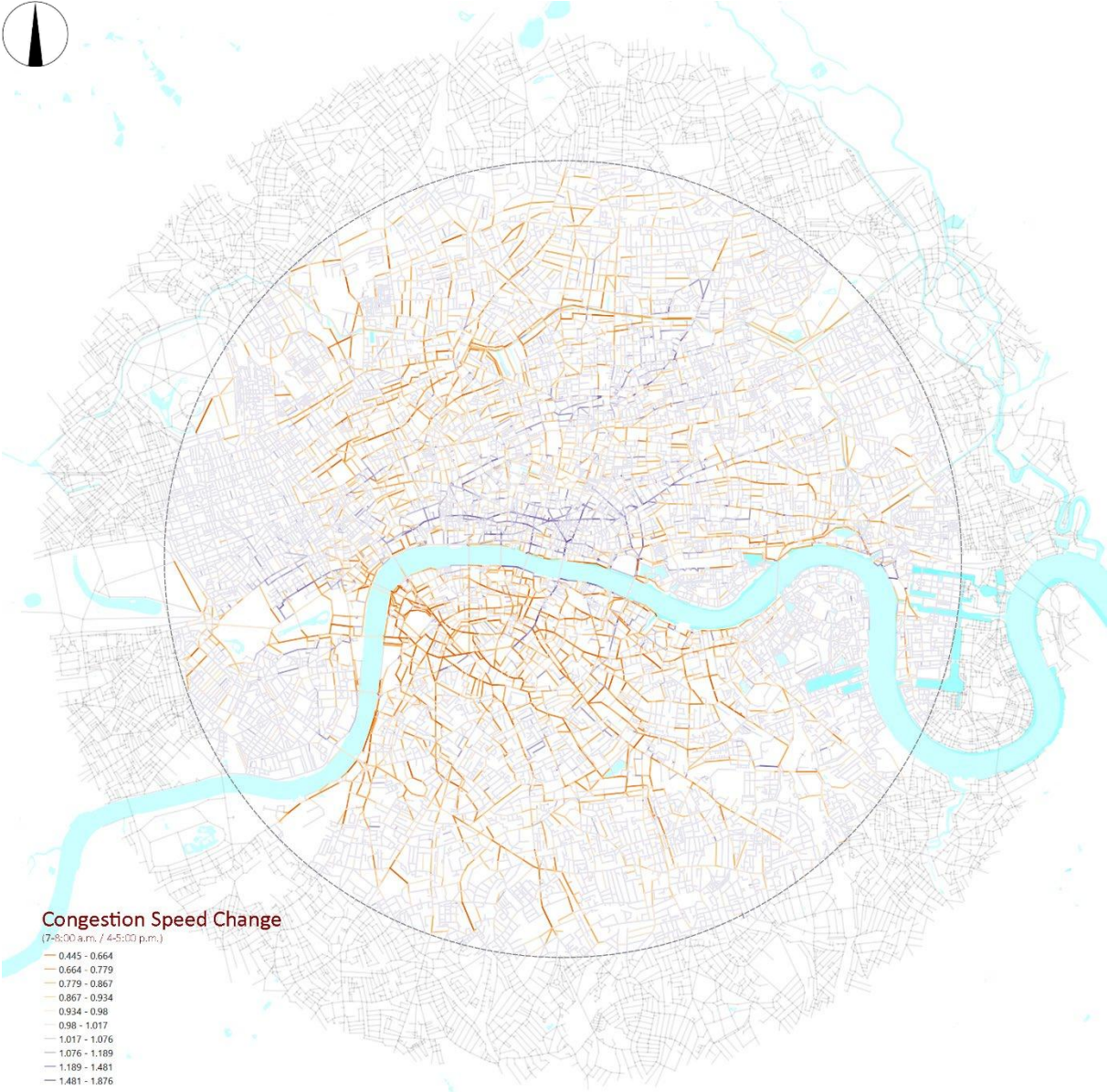
FIGURE 22 CONGESTION SPEED CHANGES BETWEEN 7-8 AM AND 4-5 PM
