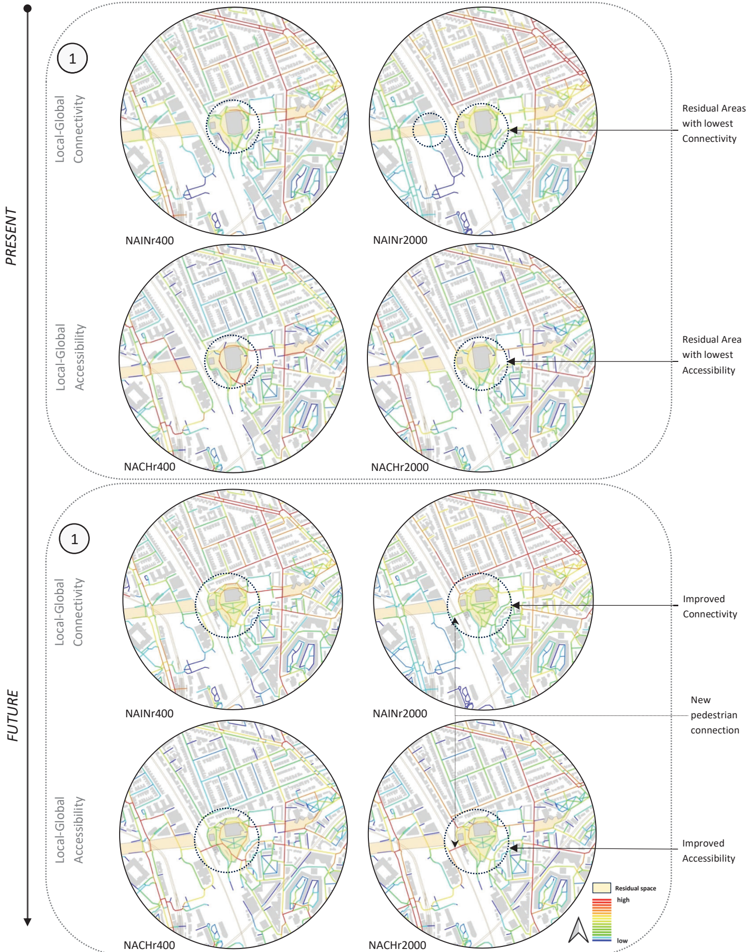
Figure 73. Set of angular segment analyses comparing present and future potential spatial configuration for Area 1.
