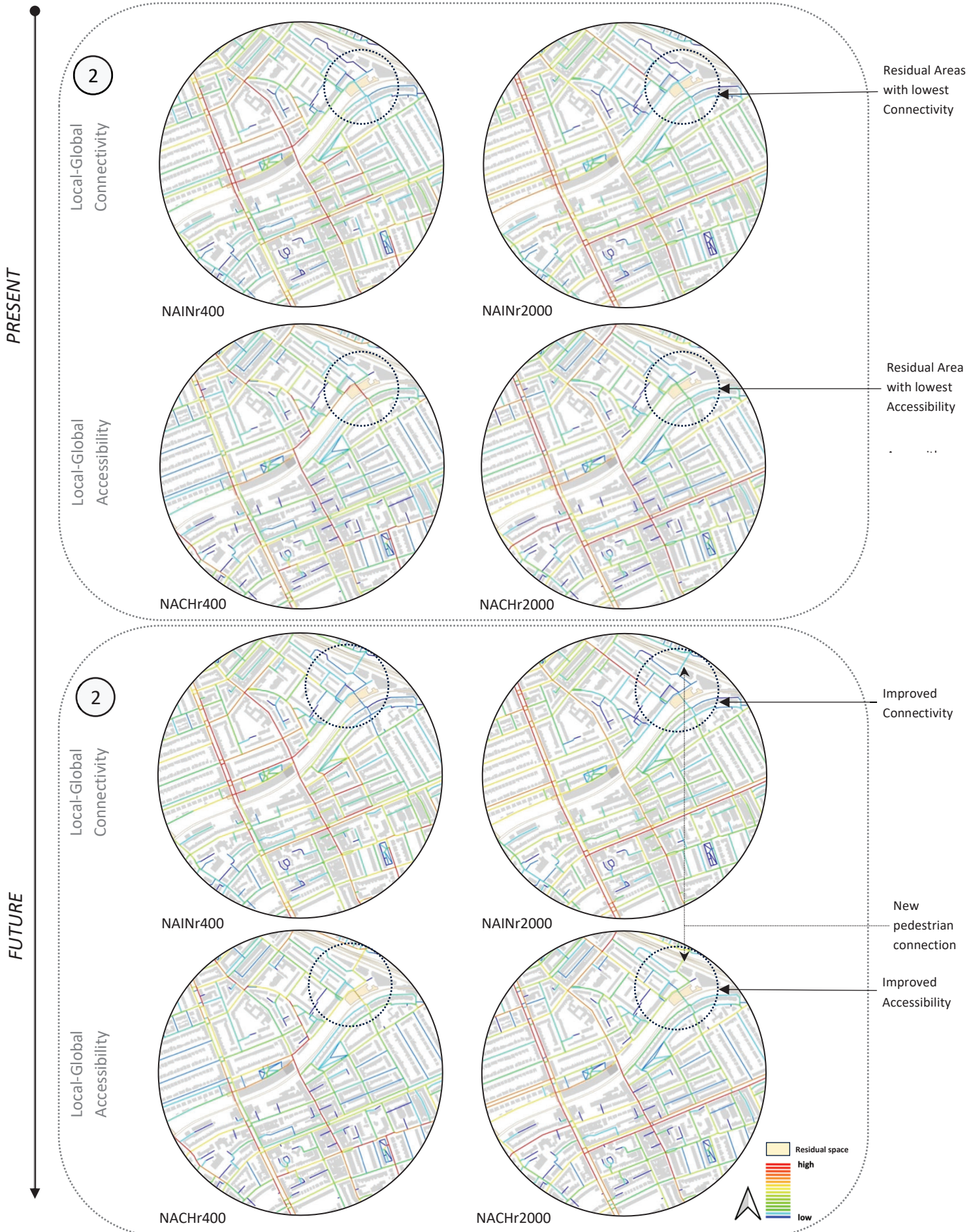
Figure 74. Set of angular segment analyses comparing present and future potential spatial configuration for Area 2.
