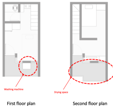
Figure 15. location of washing machine and drying space in G3.
