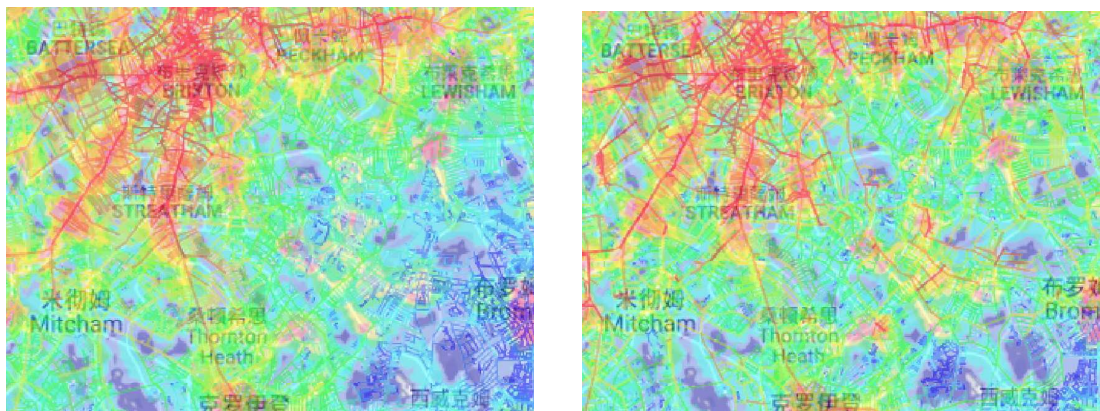
Figure 30: Overlay of PTAL map and street-based (left) and multimodal (right) global integration on the South of the Thames
