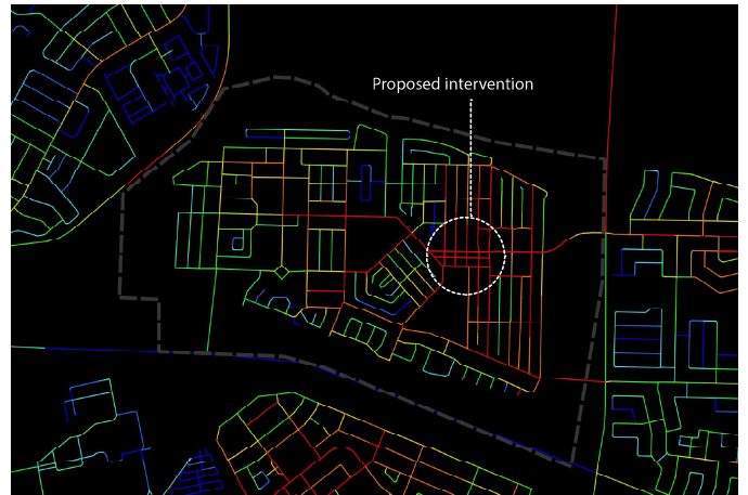
Figure 4: Angular Segment Analysis R800, of Langa with proposed design layout of its taxi rank
