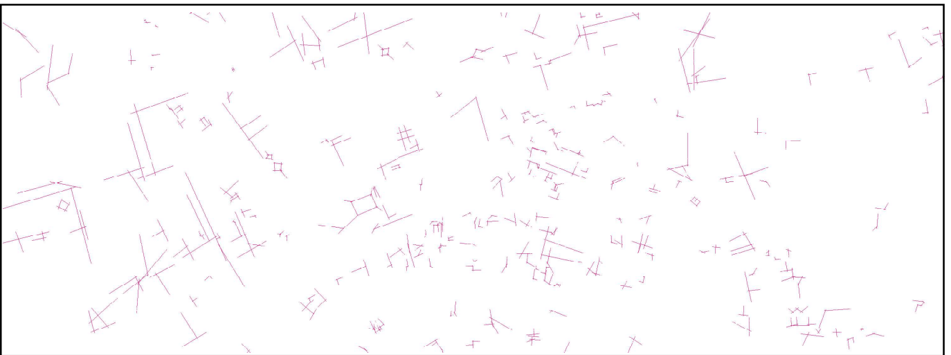
Figure A-5 These intersecting axial lines have the difference on integration R10 values more than 8% of their average.
