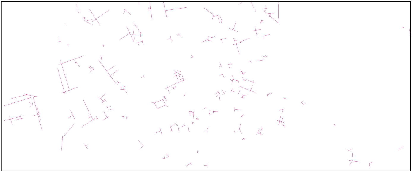
Figure A-6 These intersecting axial lines have the difference on integration R10 values more than 10% of their average.
