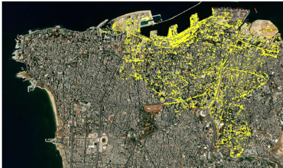
Figure 4.1: "Severe Damages" Class extracted following the Random Forest classification with the Sieve filter applied, and projected on the Optical Satellite image downloaded from Maxar dated 31st July.
