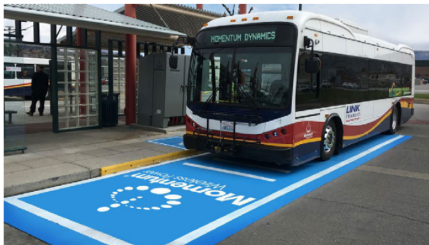
Fig. 2.9: Momentum's 200 kW wireless charging system in Wenatchee. Source: Ridden, 2018.
