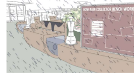
Figure 93. "Rain catcher" bench and bioretention basin can harvest and store stormwater on flooding days
