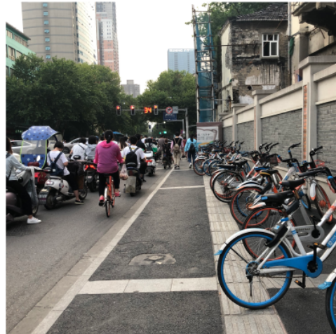
Figure 13 and 14. Vehicles occupying on the tactile paving (Author, 2019).
