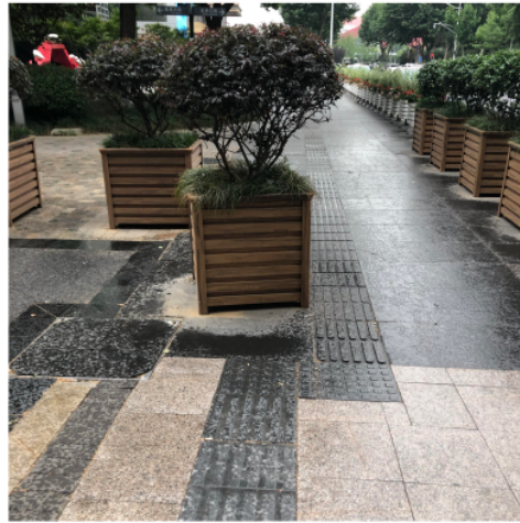
Figure 9, 10 and 11. Tactile paving impeded by other municipal facilities (Author, 2019).
