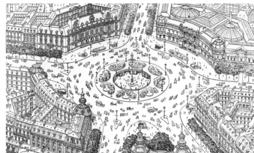
Figure 10 - Henard's traffic innovations, the roundabout (right) and an early diamond interchange (left). Note how well, despite the scale, this integrates into the urban fabric.
