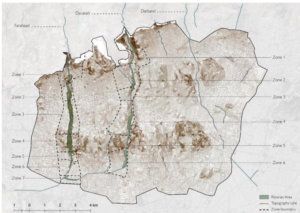
Figure 4.5 Riparian areas identified by tracking the turning points of the contour lines onto where it meets the street segment network. Author
