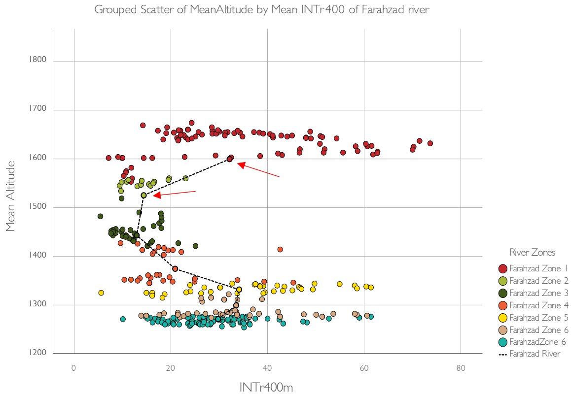
Chart 10. Combined Scatter Gram of Farahzad river zones with respect to the segments' Mean Altitude and Integration value. The dashed line represents the river itself. Author
