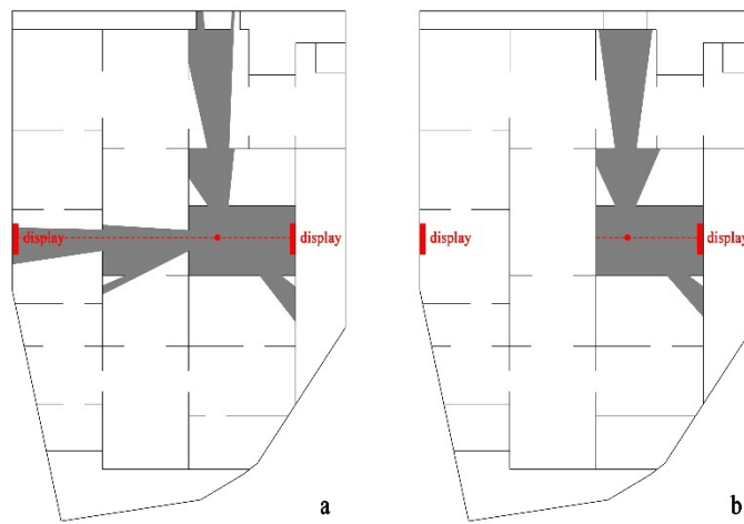
Figure 6.5: Isovist analysis showing the view of visitors in the exhibition room. (a) before reopening, (b) after reopening.
