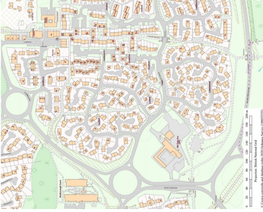
Figure 13: Ashurst 3A, completed in 1978. Designed for rental or sale to encourage greater owner occupation, its layout in closes and cul-de-sacs is closer to that of private builders than previous development corporation housing.
